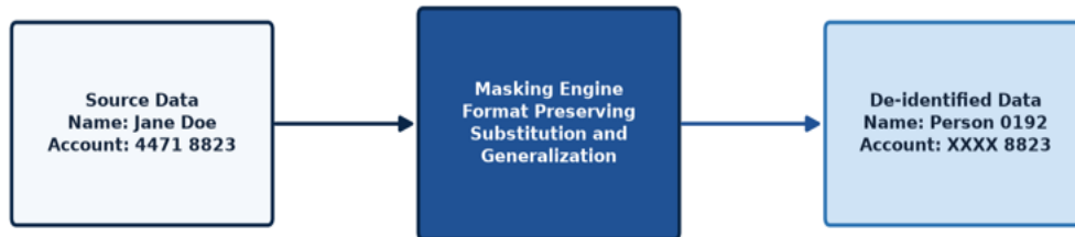
Figure 9. Data masking pipeline transforming source data into de-identified data suitable for analytics, testing, and reporting environments.
