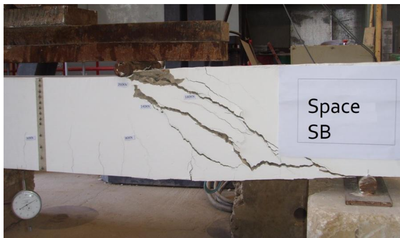
Fig. 7: Typical shear failure.
