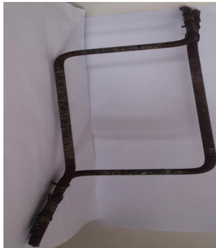
Fig. 3: Assembled space swimmer bars loop.
