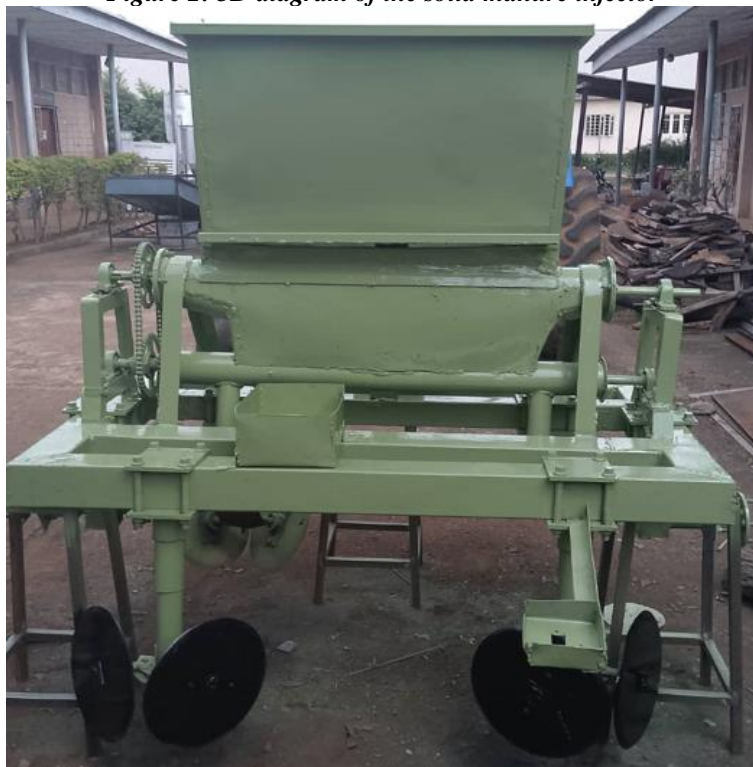
Figure 3: Fabricated solid manure injector
