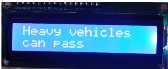
Fig 2 says, When the moisture level is above 30 and below 50 The LCD displays 'HEAVY VEHICLES CAN PASS'. At this moisture level only heavy vehicles can pass like Bus, lorries, Cargo Trucks And every vehicle can pass the Gate.
