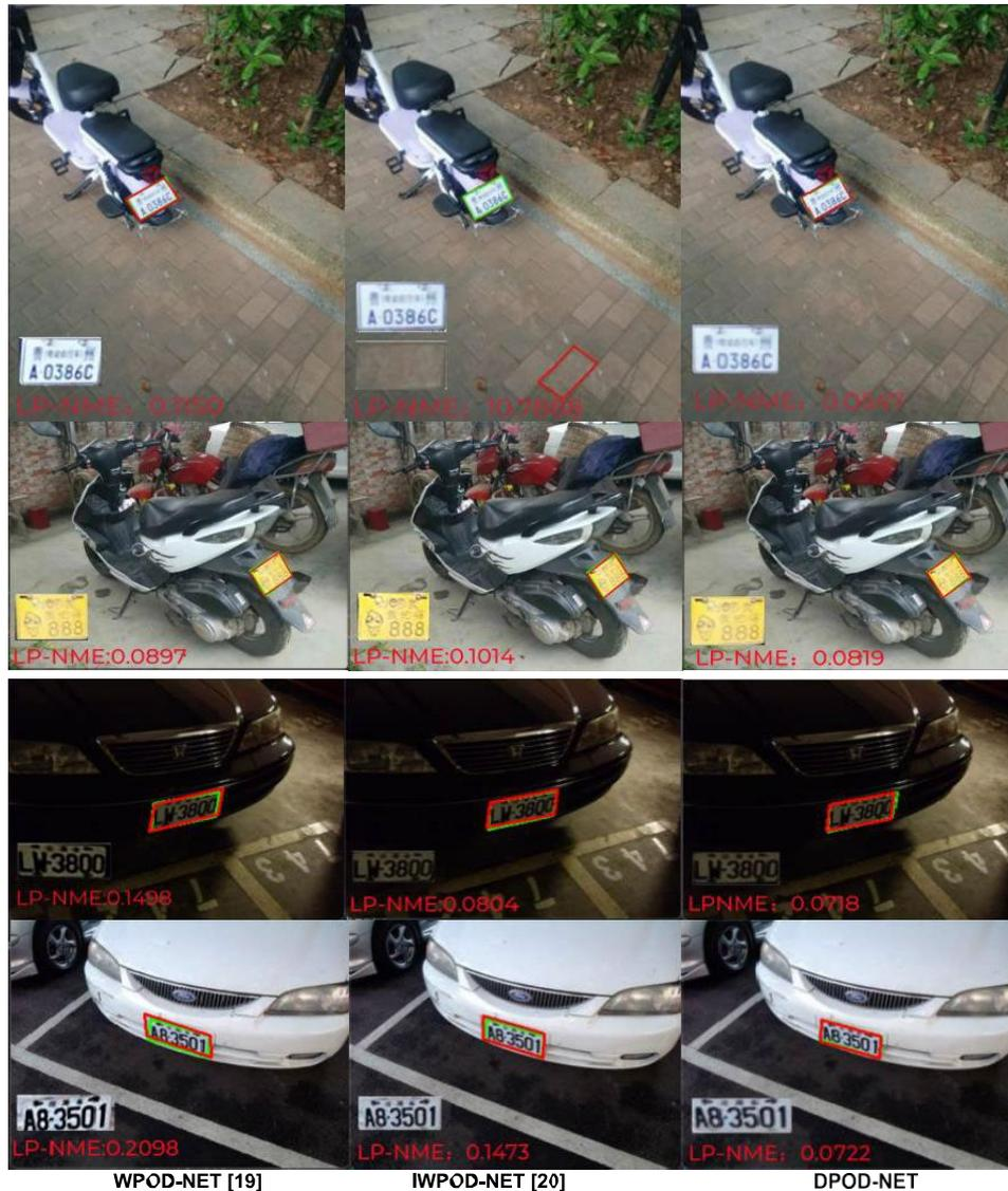
**FIG. 10.** when contrasting our method with WPOD-NET [19] and IWPOD-NET [20], the red box denotes the detection outcome, whereas the green box signifies the actual box. Values of the corrected LP and LP-NME can be located in the lower left corner of every image. This comparison utilizes images from the LPDE-4K and ALOP datasets.
