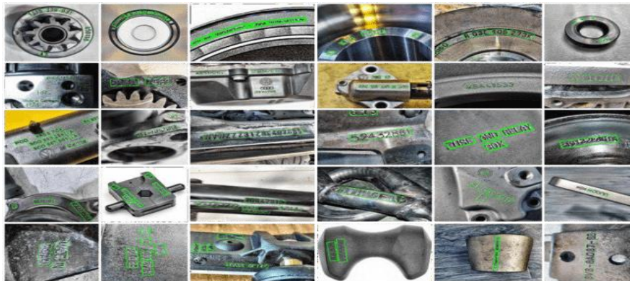
Figure 7. A few instances of multi-oriented detection using RFN on the MPSC dataset. To demonstrate how well our method for multi-oriented text identification works, five different kinds of metal components text are listed in five rows.
