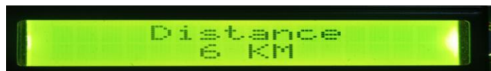
Figure (7) Distance that could be travelled with the remaining charge is displayed
