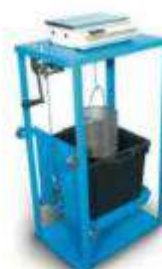
Fig. 4.1 Specific Gravity Apparatus
