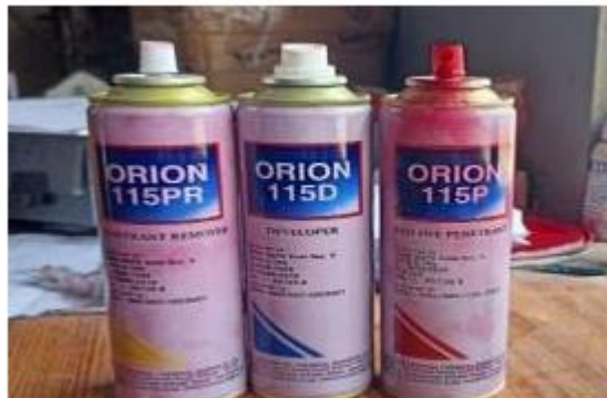
Fig.6 Dye Penetration Test
