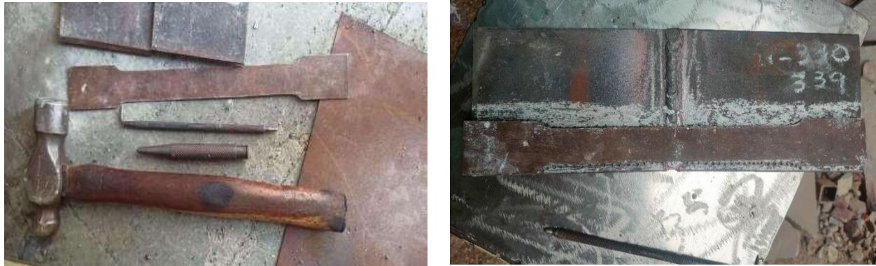
Fig.9 Marking Tools for Cutting the Specimen
