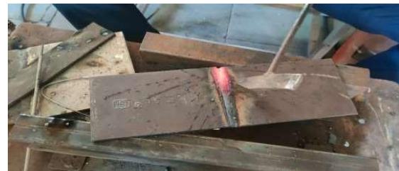
Fig.4 Shielded Metal Arc Welding on a Specimen
