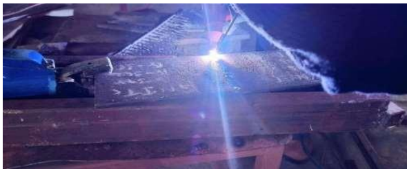
Fig.4 Shielded Metal Arc Welding on a Specimen
