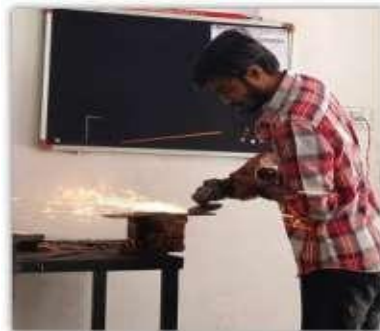
Fig.2 V-Groove Preparation by Grinding
