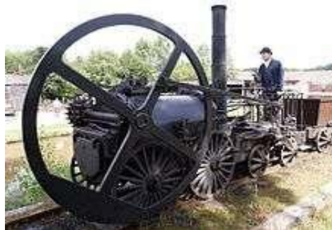
Figure 1. Flywheel to even out the power of its Single Cylinder.
