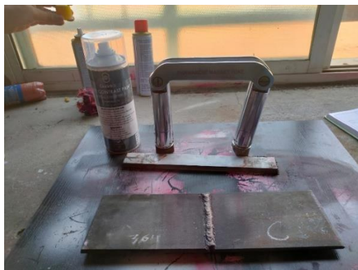
Preparation for magnetic test
