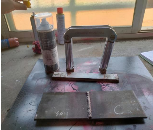
Preparation for magnetic test
