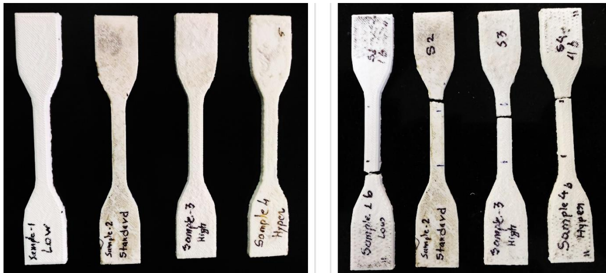
Figure 6: 3D printed ABS specimens before and after Tensile Test
