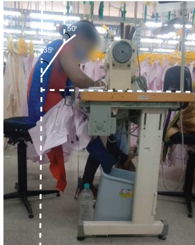
Fig 1 a: Gusset Attach operator adapting an awkward posture – angles marked for neck- trunk analysis
