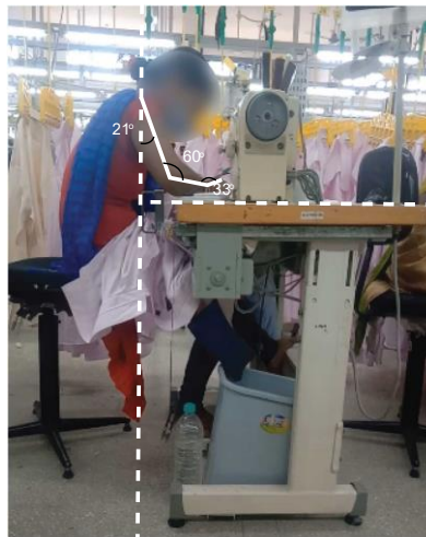
Fig 1 b: Gusset Attach operator adapting an awkward posture- angles marked for Arm- wrist analysis
