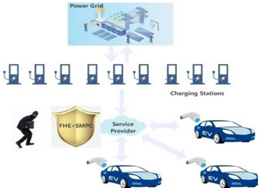
Fig 1: EV-charging station interaction system architecture [2]
