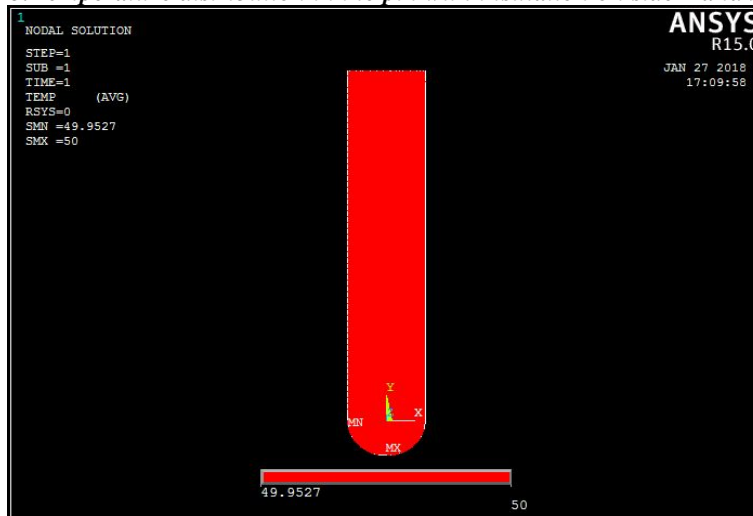
Fig. 9: Temperature distribution in the pin with insulation on side 1, side 2 and side 3
