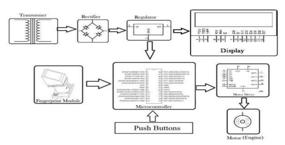
The given block diagram represents a biometric-based motor control system, likely utilizing a fingerprint module for authentication. Here's an explanation of its key components and working principle:
