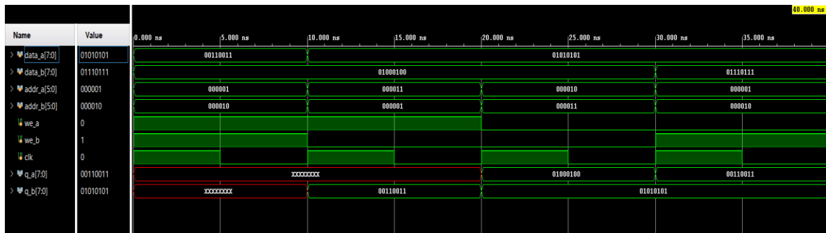
Figure 6 Waveform of read & write of Dual Port RAM
