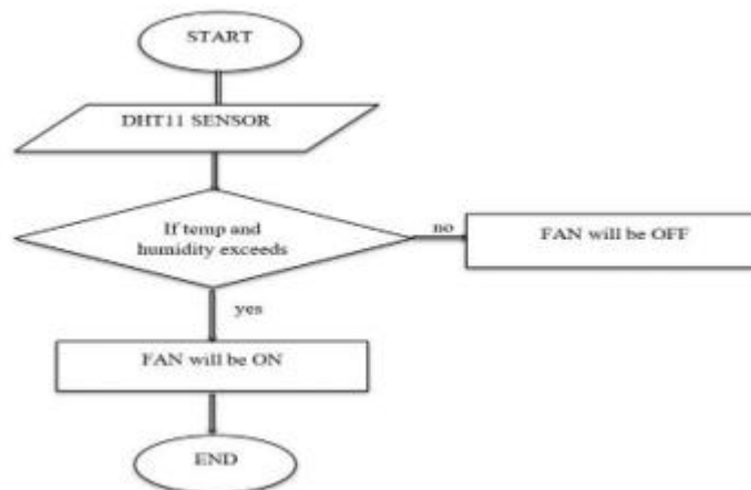
Fig 3: Flow chart of humidity detection
