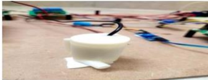
Fig 6: Interfacing Raspberry pi DC water pump
