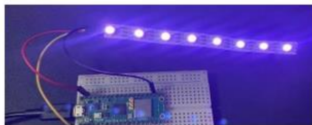
Fig 8: Interfacing Raspberry pi to LED
