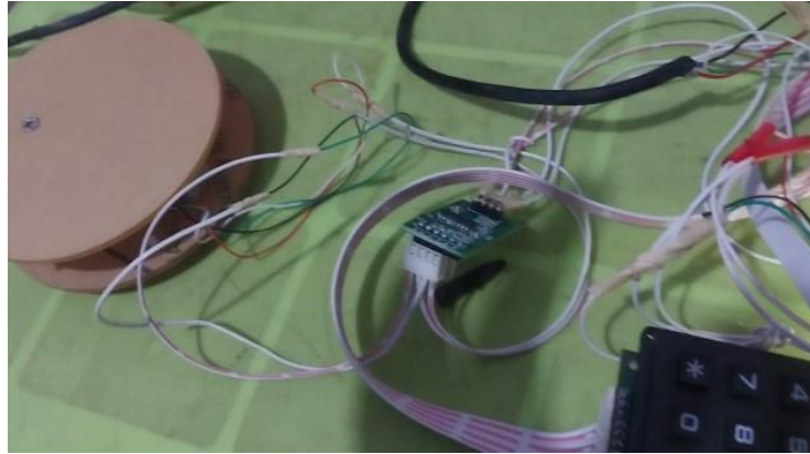
Figure 4.7: HX711 Load cell amplifier
