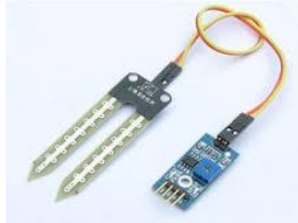
Fig.3. Soil moisture sensors
