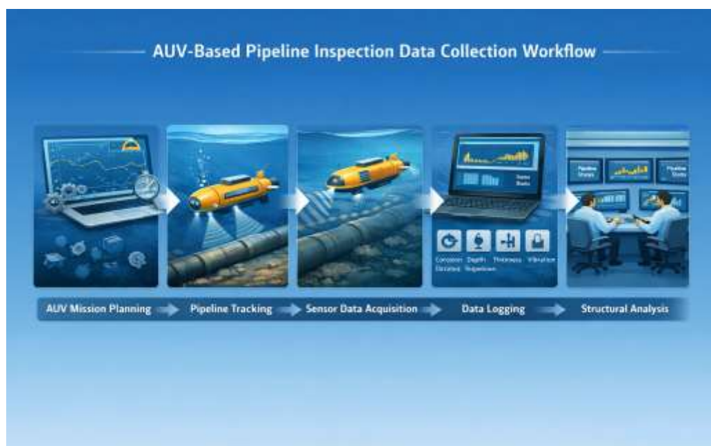
Figure 2. AUV-Based Pipeline Inspection Data Collection Workflow
