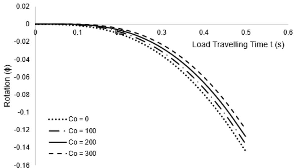
**Figure 14: Rotation of a simply supported prestressed shear beam under the action of moving load for various values of damping coefficient  $C_o$  when the Load Speed  $C = 50$  and for fixed values of  $K = 4000$ ,  $G = 4000$ ,  $N = 4000$  and  $L = 50$**
