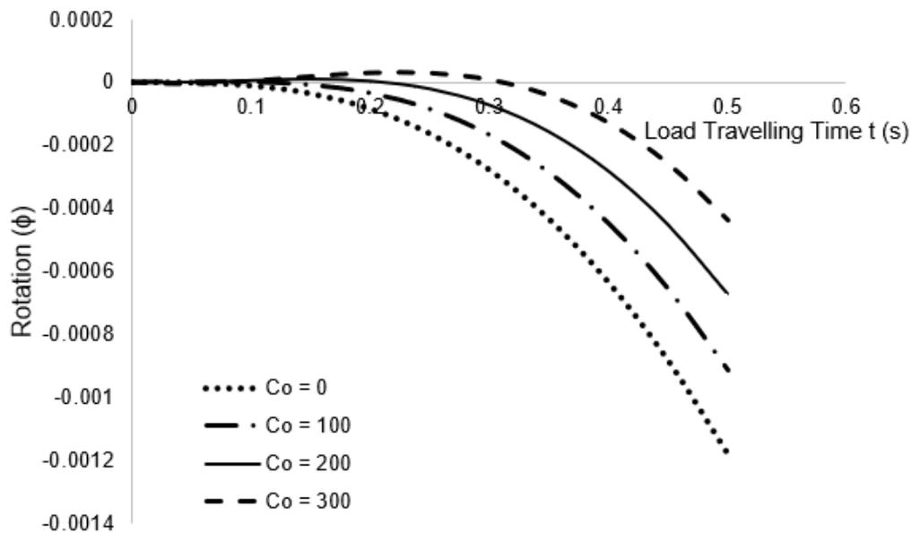
**Figure 10: Rotation of a simply supported prestressed shear beam under the action of moving load for various values of damping coefficient  $C_0$  when the Load Speed  $C = 40$  and for fixed values of  $K = 4000$ ,  $G = 4000$ ,  $N = 4000$  and  $L = 50$**
