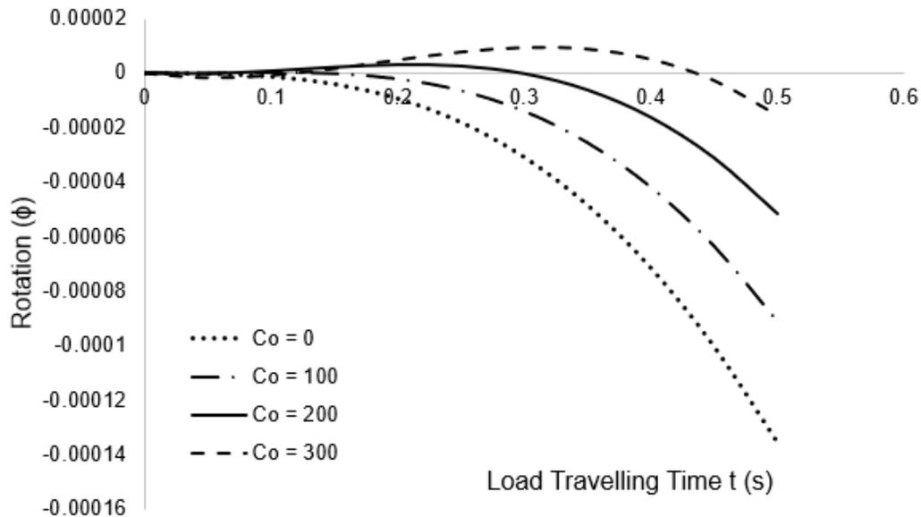
**Figure 8: Rotation of a simply supported prestressed shear beam under the action of moving load for various values of damping coefficient  $C_o$  when the beam length  $L = 65$  and for fixed values of  $K = 4000$ ,  $G = 4000$ ,  $N = 4000$  and  $C = 40$**
