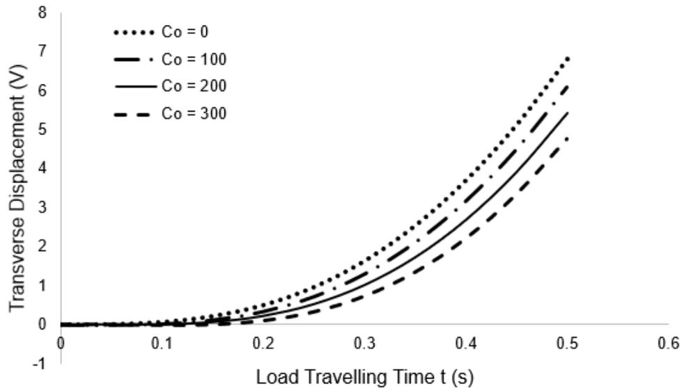
**Figure 11: Transverse displacement of a simply supported prestressed shear beam under the action of moving load for various values of damping coefficient  $C_0$  when the Load Speed  $C = 45$  and for fixed values of  $K = 4000$ ,  $G = 4000$ ,  $N = 4000$  and  $L = 50$**
