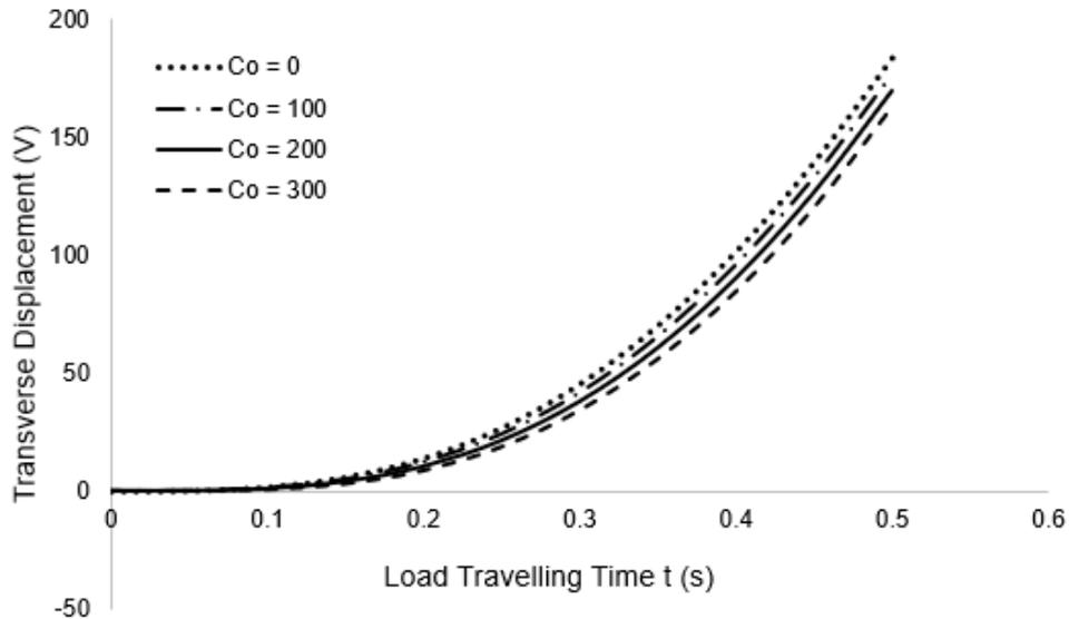
**Figure 15: Transverse displacement of a simply supported prestressed shear beam under the action of moving load for various values of damping coefficient  $C_0$  when the Load Speed  $C = 55$  and for fixed values of  $K = 4000$ ,  $G = 4000$ ,  $N = 4000$  and  $L = 50$**
