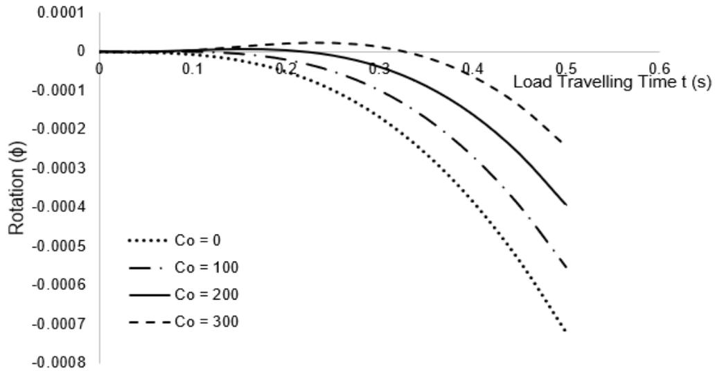
**Figure 4: Rotation of a simply supported prestressed shear beam under the action of moving load for various values of damping coefficient  $C_o$  when the beam length  $L = 55$  and for fixed values of  $K = 4000$ ,  $G = 4000$ ,  $N = 4000$  and  $C = 40$**
