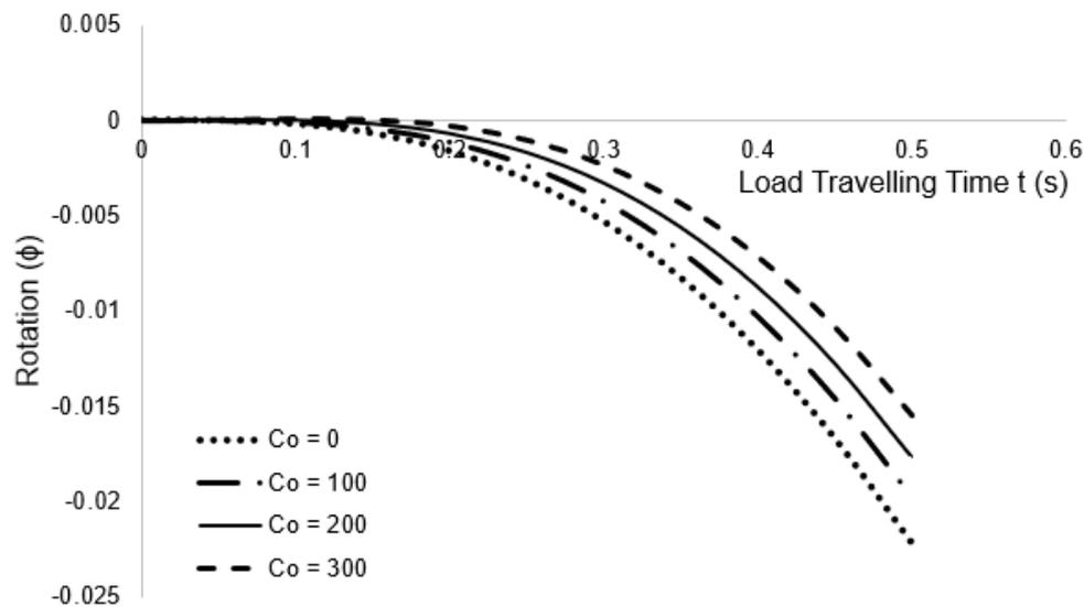
**Figure 12: Rotation of a simply supported prestressed shear beam under the action of moving load for various values of damping coefficient  $C_0$  when the Load Speed  $C = 45$  and for fixed values of  $K = 4000$ ,  $G = 4000$ ,  $N = 4000$  and  $L = 50$**
