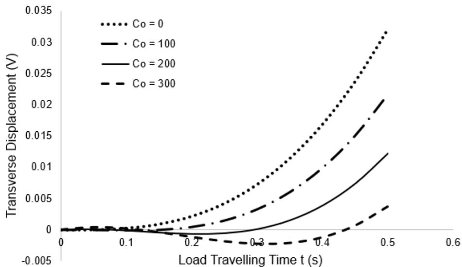
**Figure 7: Transverse displacement of a simply supported prestressed shear beam under the action of moving load for various values of damping coefficient  $C_o$  when the beam length  $L = 65$  and for fixed values of  $K = 4000$ ,  $G = 4000$ ,  $N = 4000$  and  $C = 40$**
