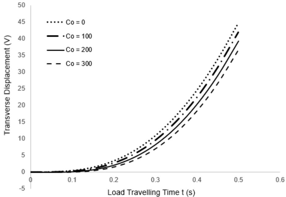
**Figure 13: Transverse displacement of a simply supported prestressed shear beam under the action of moving load for various values of damping coefficient  $C_o$  when the Load Speed  $C = 50$  and for fixed values of  $K = 4000$ ,  $G = 4000$ ,  $N = 4000$  and  $L = 50$**
