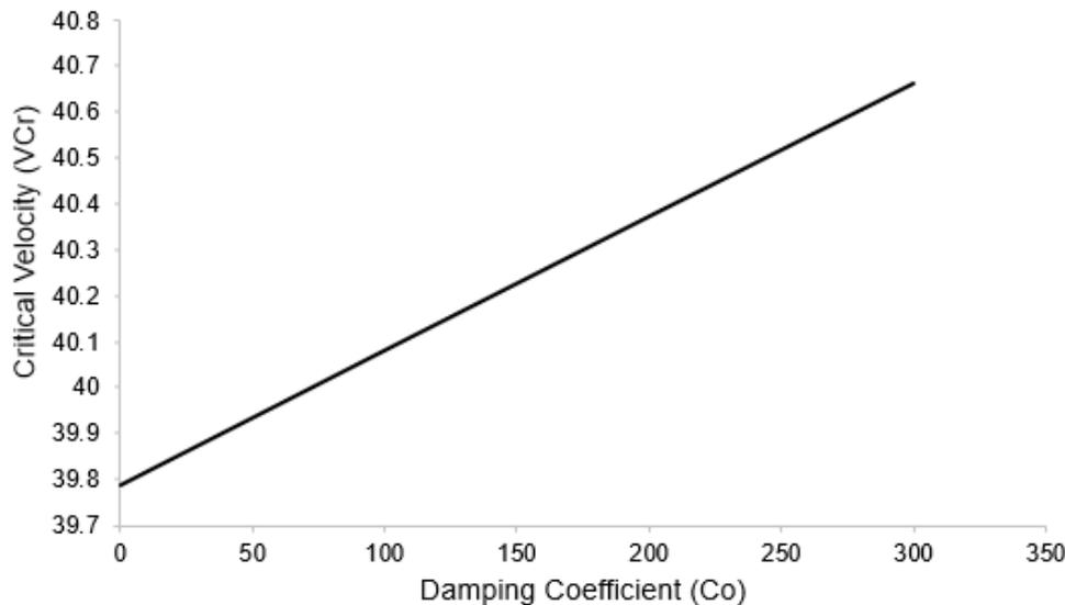
*Figure 17: Variation of the critical velocity ( $V_{Cr}$ ) against damping coefficient ( $C_0$ )*
