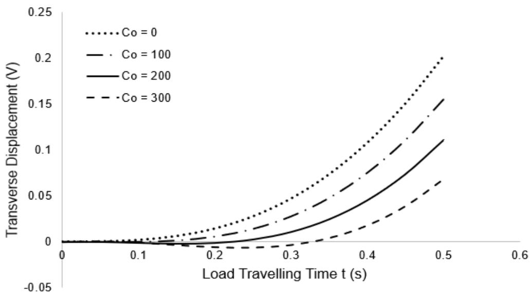
**Figure 3: Transverse displacement of a simply supported prestressed shear beam under the action of moving load for various values of damping coefficient  $C_o$  when the beam length  $L = 55$  and for fixed values of  $K = 4000$ ,  $G = 4000$ ,  $N = 4000$  and  $C = 40$**
