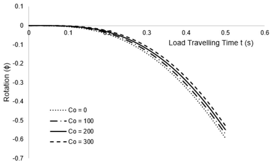
**Figure 16: Rotation of a simply supported prestressed shear beam under the action of moving load for various values of damping coefficient  $C_0$  when the Load Speed  $C = 55$  and for fixed values of  $K = 4000$ ,  $G = 4000$ ,  $N = 4000$  and  $L = 50$**
