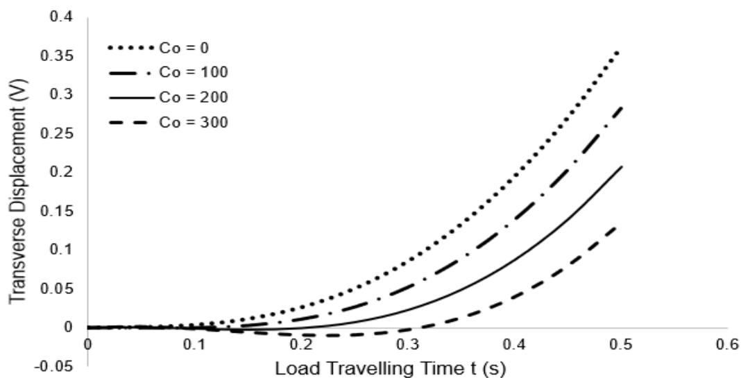
**Figure 1: Transverse displacement of a simply supported prestressed shear beam under the action of moving load for various values of damping coefficient  $C_o$  when the beam length  $L = 50$  and for fixed values of  $K = 4000$ ,  $G = 4000$ ,  $N = 4000$  and  $C = 40$**
