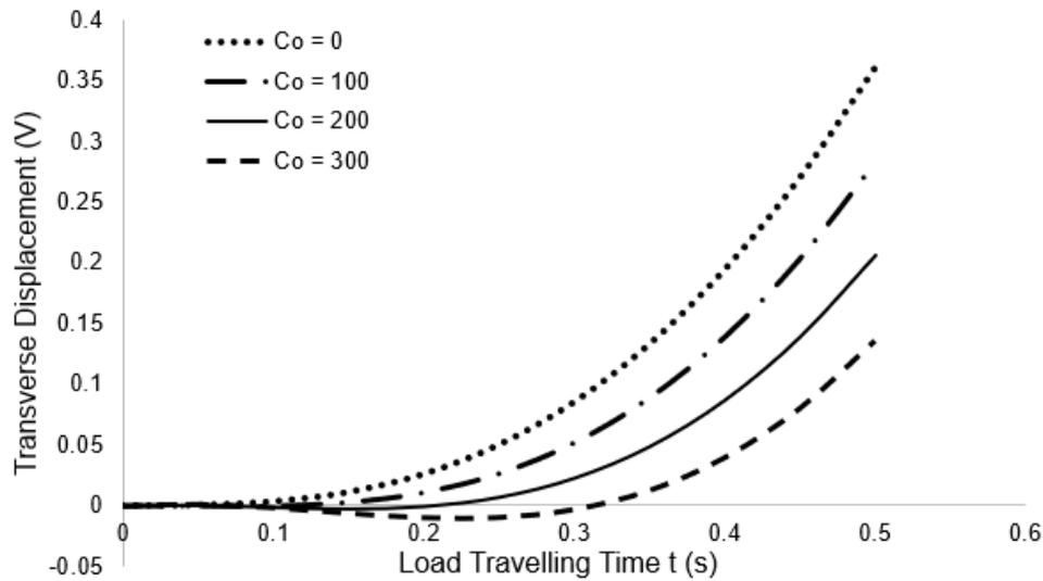
**Figure 9: Transverse displacement of a simply supported prestressed shear beam under the action of moving load for various values of damping coefficient  $C_0$  when the Load Speed  $C = 40$  and for fixed values of  $K = 4000$ ,  $G = 4000$ ,  $N = 4000$  and  $L = 50$**
