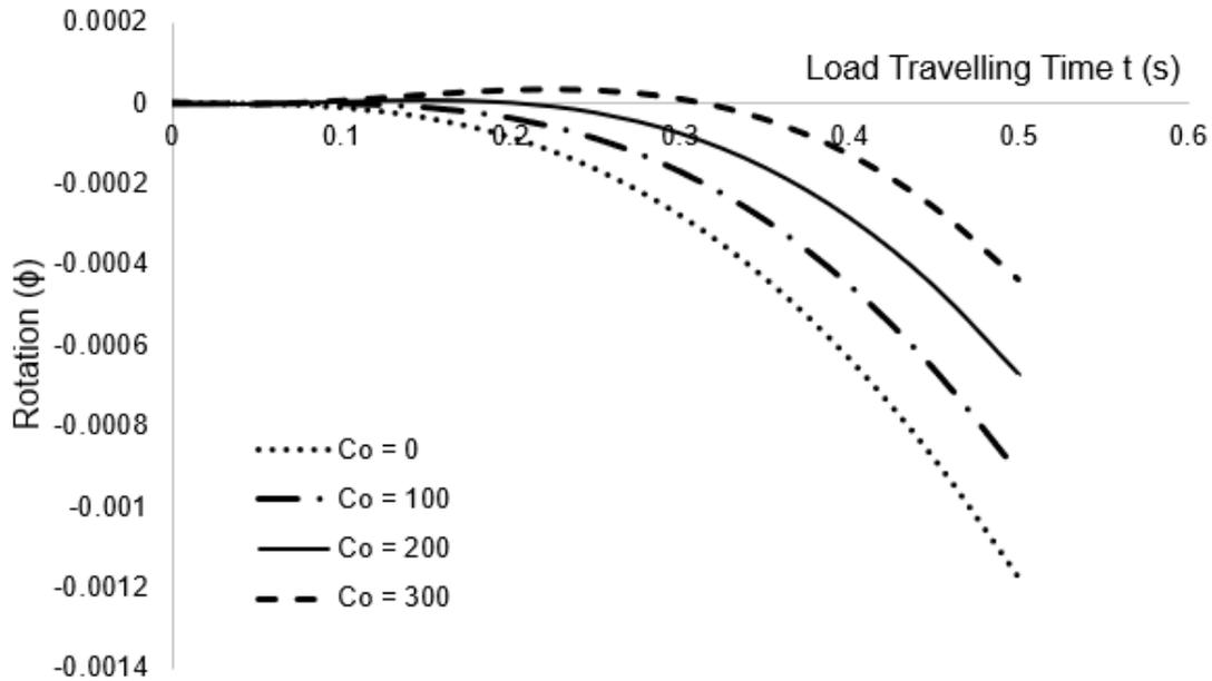
**Figure 2: Rotation of a simply supported prestressed shear beam under the action of moving load for various values of damping coefficient  $C_o$  when the beam length  $L = 50$  and for fixed values of  $K = 4000$ ,  $G = 4000$ ,  $N = 4000$  and  $C = 40$**
