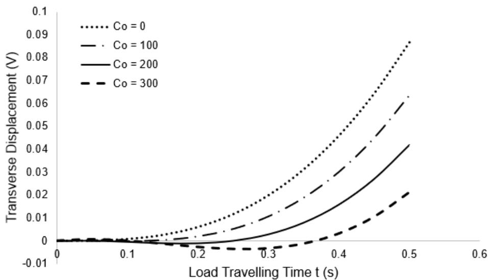
**Figure 5: Transverse displacement of a simply supported prestressed shear beam under the action of moving load for various values of damping coefficient  $C_o$  when the beam length  $L = 60$  and for fixed values of  $K = 4000$ ,  $G = 4000$ ,  $N = 4000$  and  $C = 40$**
