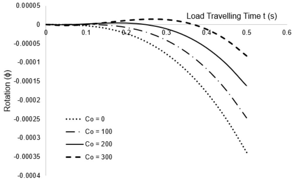
**Figure 6: Rotation of a simply supported prestressed shear beam under the action of moving load for various values of damping coefficient  $C_o$  when the beam length  $L = 60$  and for fixed values of  $K = 4000$ ,  $G = 4000$ ,  $N = 4000$  and  $C = 40$**
