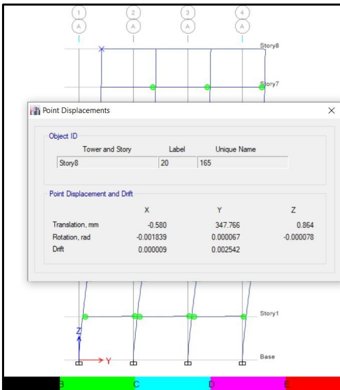
Hinge Formation for SRC Rectangular Building with opening (X direction) Hinge Formation for RCC Rectangular Building with opening (Y direction)
