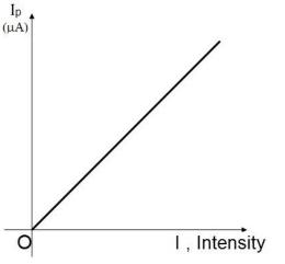
verification of photoelectric current
