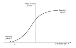
effect of potential on photoelectric current
