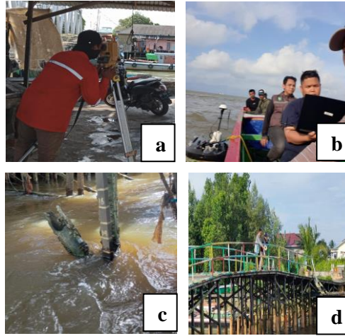
Figure 1. Main Surveys a. Topological survey. b. Bed bathymetry survey. c. Peil scale for observation. d. River flow discharge measurement
