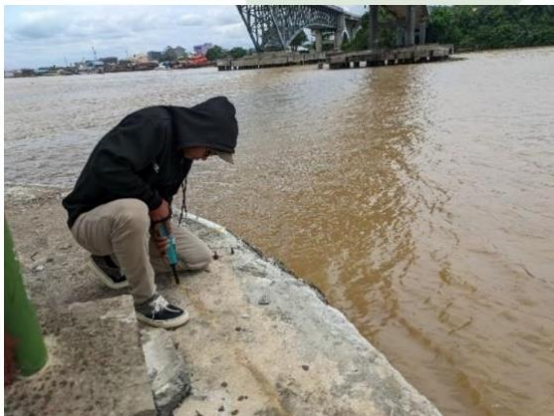
Figure 10. Concrete insitu test points taken at P3 pillar
