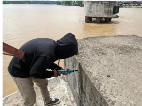
Figure 10. Concrete insitu test points taken at P3 pillar
