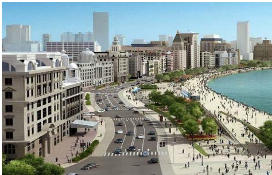
Figure 9. Increasing the width of the platform and reducing the number of car lanes it gives a sense of security. [Source: Xin Min, 2011, P43].
