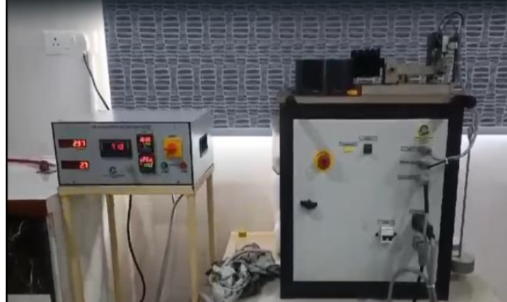
Fig. 7 Pin on Disc Wear Test of 3D printed samples
