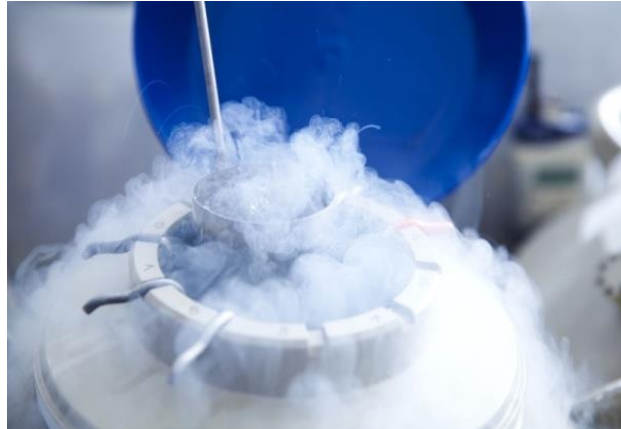
Fig. 5 Deep Cryogenic treatment of 3D printed test samples
