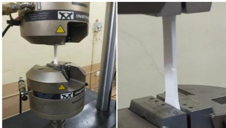
Fig. 6 Tensile Testing of 3D printed samples
