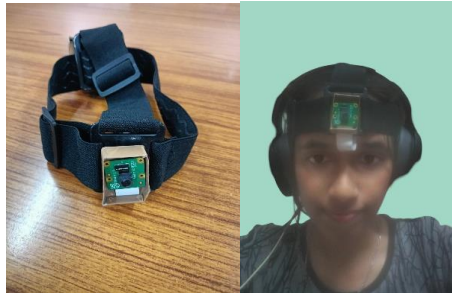
Fig. 2. Experimental setup with the raspberry pi camera attached to the front end of the GoPro and the raspberry pi CM4 on its rear end. This device is light and easy to wear by the user.
