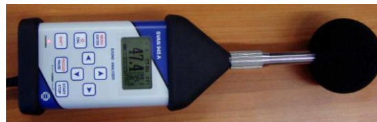
Fig. 3. View of the meter of the acoustic pressure level.
