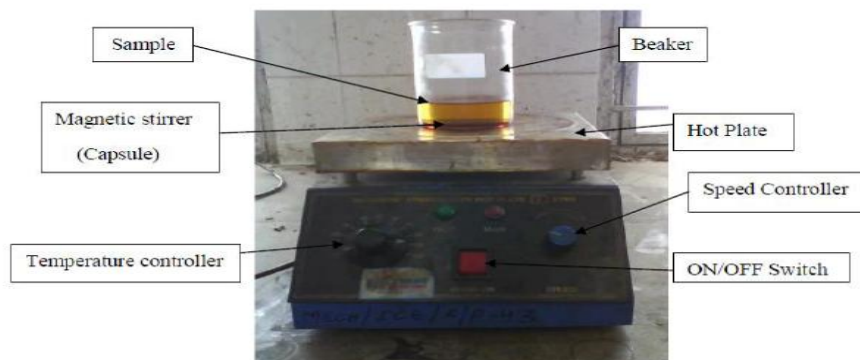
Fig 1: Experimental set-up of biodiesel reactor with mechanical stirrer
