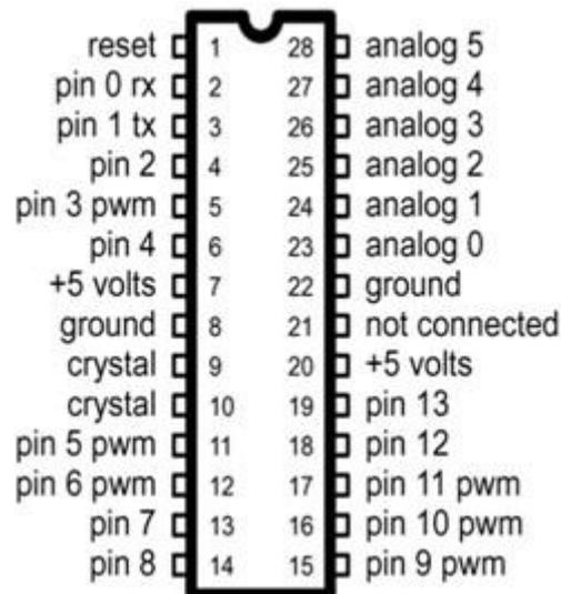
Fig.3: Pinout of the Atmega328
