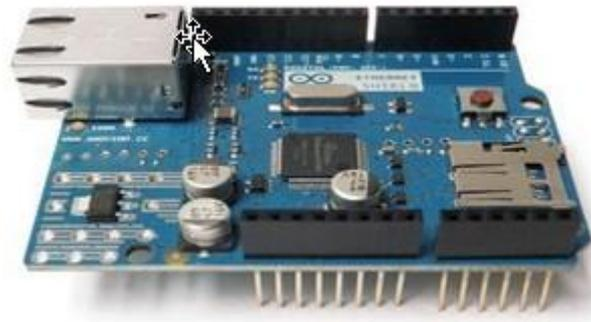
**Fig. 5: Ethernet Shield**
