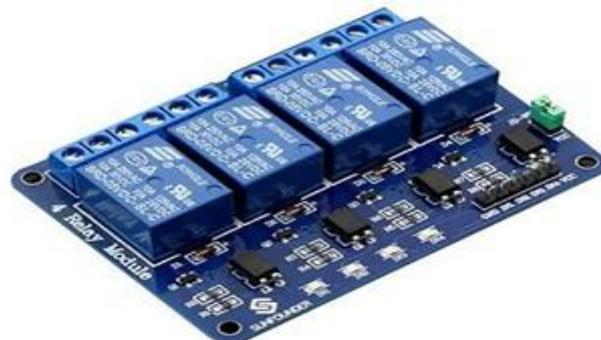
*Fig. 6: 4 Channel Relay board*
