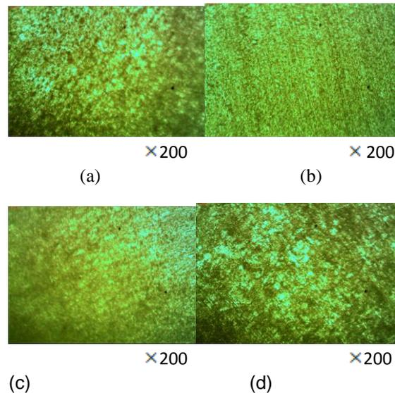
*Fig. 1: Micro-structure of mild steel samples (a) as received, (b) quenched in air, (c) quenched in water and (d) quenched in engine oil*
