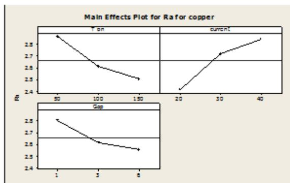
*Fig.8 : The Effect of current, pulse on Time and Gap on ( Ra) using copper electrode.*
