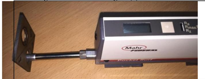
*Fig.6 : Automatic digital POCKET SURF EMD-1500.*
