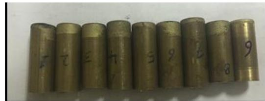
*Fig.4 : shown brass electrode after cutting process*
