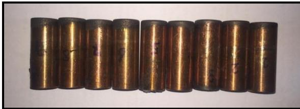
*Fig.3 : shown copper electrode after cutting process*
