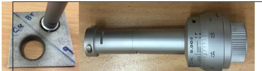
*Fig.7 : Micrometer used for hole.*
