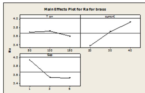
*Fig.9 : The Effect of current, pulse on Time and on (Ra) using Brass electrode.***Effect of Electrode Material on Diameter Error (Ed)**
